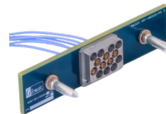
VITA 67.3 RF VPX modular connection system
