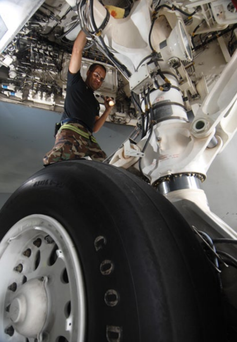
▲ Aircraft wheel wells are a particularly challenging environment for EWIS routing
