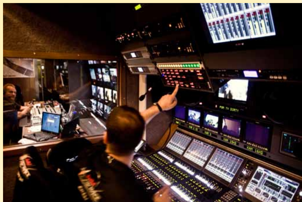
On board the SIVision High-Definition mobile broadcasting unit—a “control room on wheels” for audio and video electronic field production.
