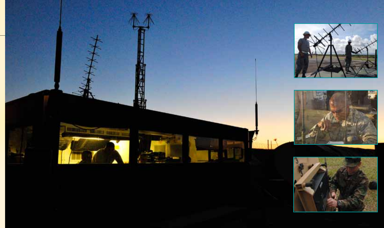
Main Photo: Command and control specialists work inside a Mobile Air Reporting Communications shelter at Camp Marmal, Afghanistan. The MARC is an air-deployable mobile tactical shelter that provides CRW Airmen with the ability to communicate with aircraft as well as schedule and track cargo movements worldwide. Inset Photos: Mobile tactical shelter specialists installing rooftop antennae, working inside a shelter, and checking communications equipment.
