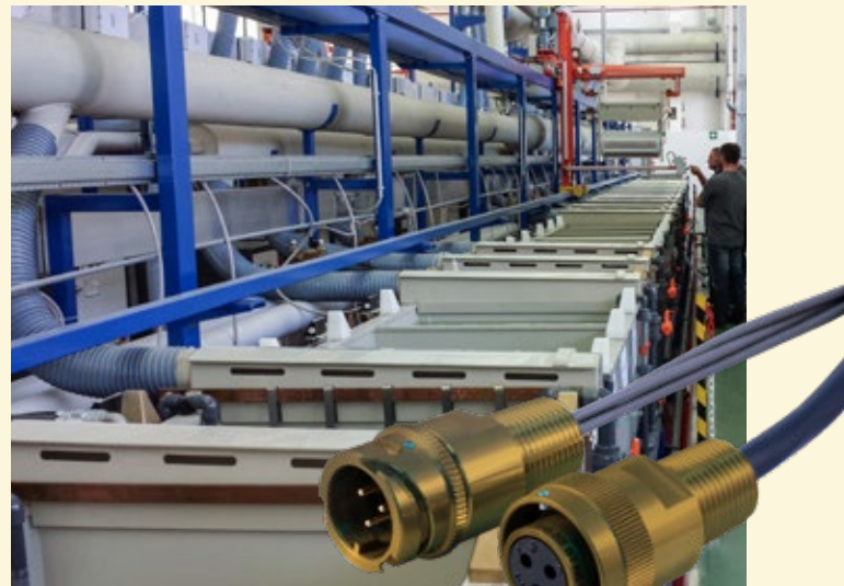
ADVANCED PLATING LINE Capabilities include VG95328-qualified Marine Bronze and "Code J" Tin-Zinc plating—VG95211 and VG95212 qualified cadmium alternative for corrosion-resistant interconnects.
