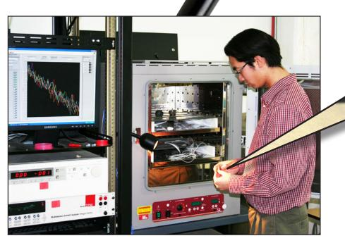
Glenair's state-of-the-art diode burn in process tests leaded and surface mount diodes with leakage current monitored throughout the entire test procedure, ensuring field reliability.
