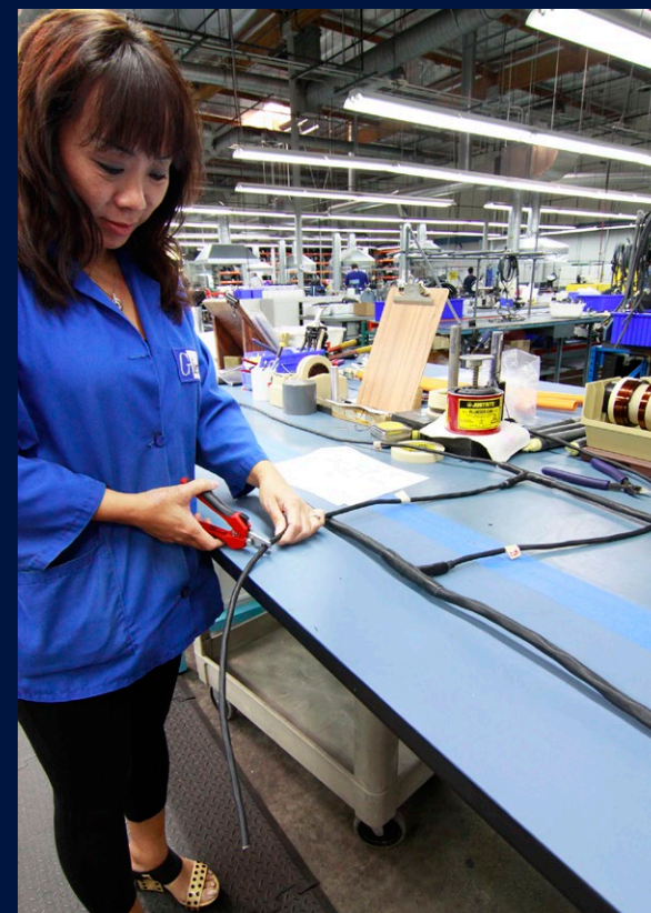
▶ Skilled technicians produce made-to-measure multi-branch assemblies to exact dimensional tolerances
