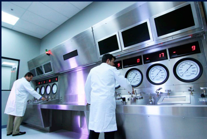
Glenair's hydrostatic test lab control room: modular consoles provide for up to 8 pressure circuits, operating in manual or automated mode. Each circuit is capable of a maximum of 16.5K psi.
