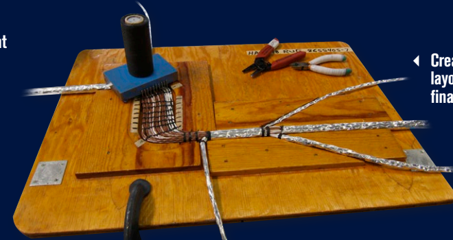
▶ Skilled technicians produce made-to-measure multi-branch assemblies to exact dimensional tolerances
