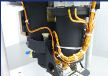
Harness integration into space payload electromechanical devices
