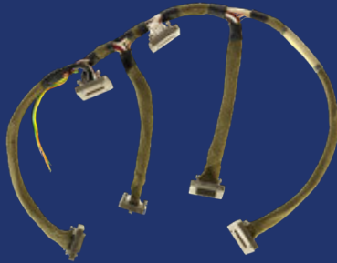
Multibranch wire harness with Glenair Micro-D connectors
