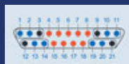
High-Speed Micro-D TwistPin contact 10+Gb/sec. (example insert with four high-speed signal pairs)
