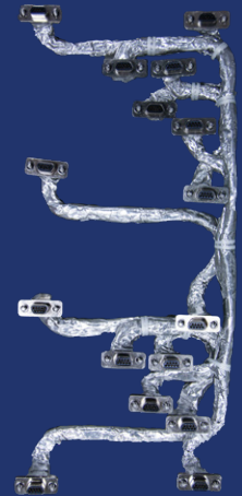
Mylar tape-wrapped assembly with Glenair Micro-D connectors
