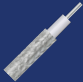
Size 047 26.5 GHz hand-formable tin-soaked braid
